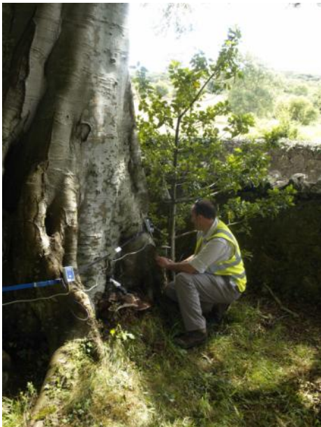
Surveyor undertaking a Picus survey of a diseased beech tree in a churchyard in Penrtraeth
